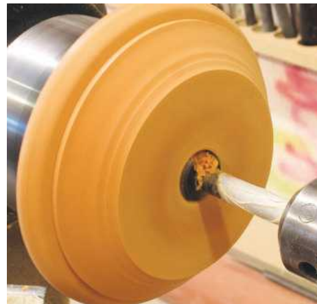
▲ Pic.12 Before doing the shaping on the top, drill a 30mm stem hole with a saw-tooth bit. Slow the lathe down to about 400rpm when doing this
